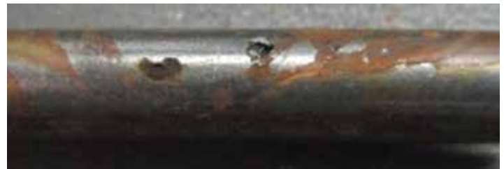
Figure 7: Pitting with related staining on 420 stainless Slotted Pin.
