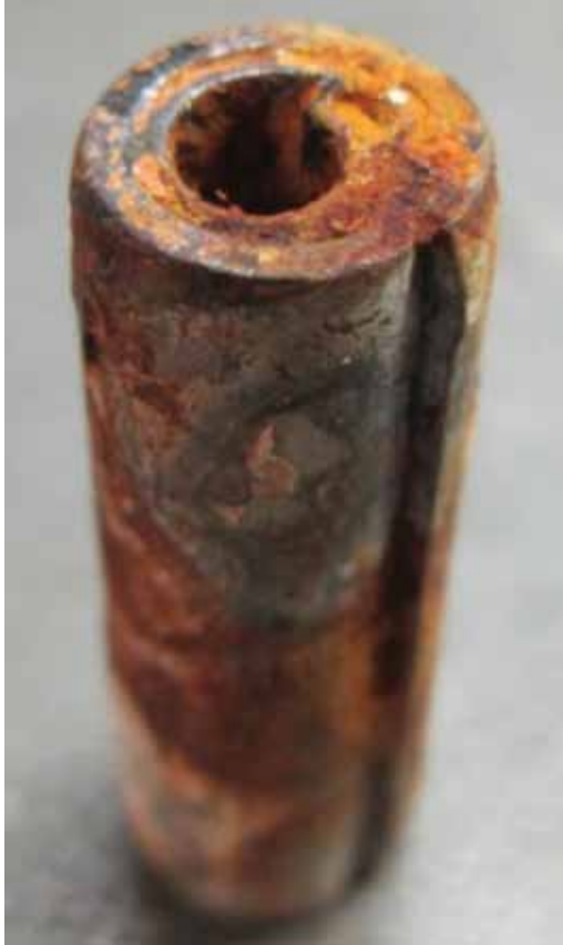
Figure 3: This photograph demonstrates the basic geometry of a Coiled Pin – it consists of a number of metal wraps. Platings will not penetrate between the wraps and dip coatings, though capable of covering the interior, will remain ineffective between the pin's wraps.
