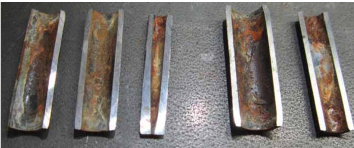
Figure 4: To demonstrate attack between the Coiled Pin's coils (or wraps) of steel, the photograph below was taken after cross-sectioning the pin shown in Figure 3.
