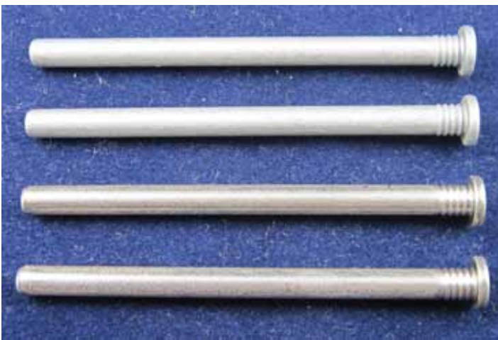
Figure 5: Pins prior to test: the top two are low carbon steel coated with zinc lamellar, the bottom two are austenitic 305 SST.
