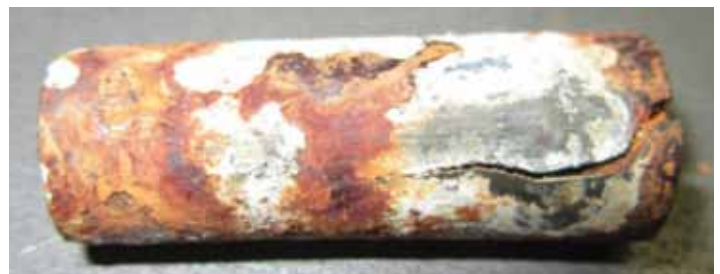
Figure 2: This Coiled Pin was finished with a light duty zinc plating and subsequent chromate dip. The finish was rated for 48 hours to 'red' corrosion protection. Leaving this item in salt spray for 200 hours has resulted in significant red rust though some zinc and white corrosion remain. Where zinc is present on the surface, the part remains free of red rust despite the severity of attack in adjacent areas.
