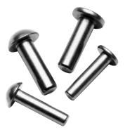
In order to utilize traditional automating methods, headed parts should be able to hang by the head. A good rule of thumb is that there should be a minimum of a 20% differential between the head and body diameter in order to provide enough distinction to allow for orienting and hanging If the diameter the parts. differential can be held
