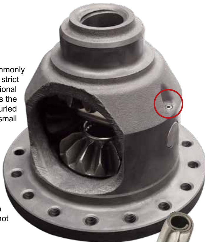
SPIROL Coiled Spring Pin retains a pinion shaft in a differential carrier assembly.
