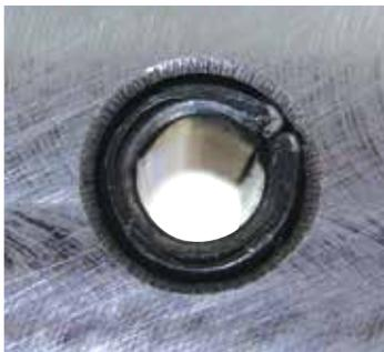
Figure 2. The Slotted Pin's gap is closed when installed in a hole.
