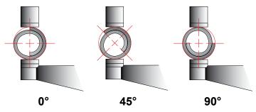
Figure 4. Micrometer measurements.
