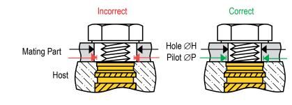
Hole in mating part must be smaller than Insert pilot diameter in host to prevent the Insert from pulling through the assembly – known as "jack-out".
