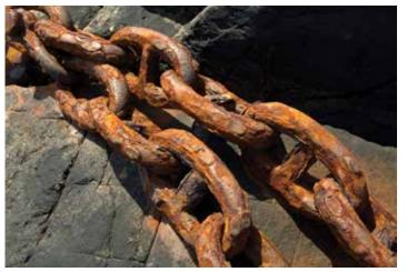
Rust occurs in iron and iron alloys such as steel. Rust is a layer of iron oxide created at the surface of a part when exposed to oxygen in the presence of moisture. This layer of iron oxide remains active and continues to convert iron to iron oxide as the outer layers lose integrity and fall away exposing new metal (See Figure 1). Iron oxide is also porous allowing it to absorb moisture and elements that may contribute
