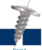
Figure 4 Misaligned Screw
