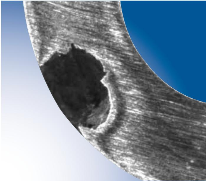
Figure 1. Cross section of pit demonstrating impact on cross-sectional area and reduction in strength
