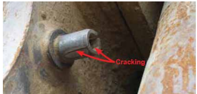
Figure 3: A Slotted Pin can only flex along its spine 180° opposite the gap, much like opening and closing a book.
