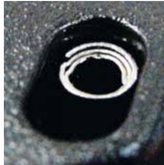
Figure 4. Using an improper installation tool will make the pin telescope or unwrap.
