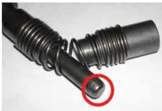
Figure 3. Worn insertion quill
